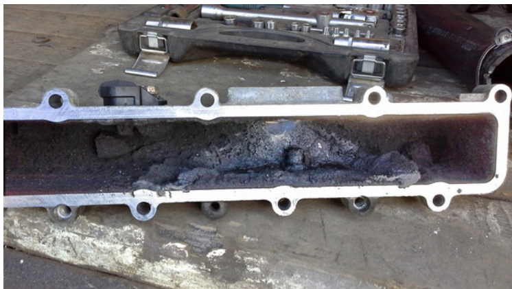
Soot build up inside Iveco F1C Plenum - inlet manifold , EGR error 148.
