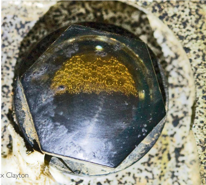
oil foaming in sight glass
