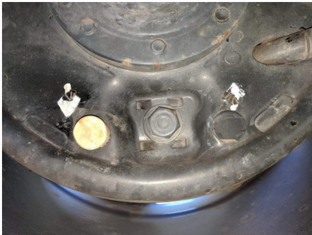
Left side , and right side rear backing plates, note new rear shoe adjuster holes with corks
