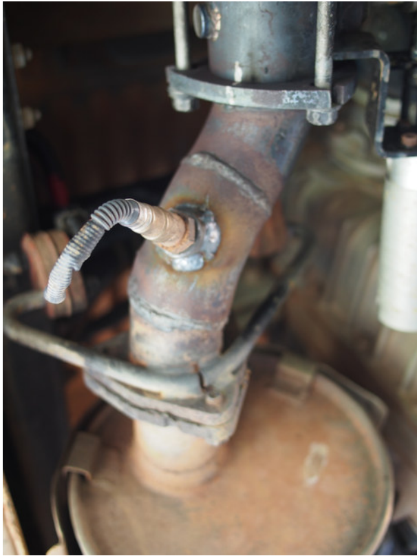
relocated Lambda sensor
