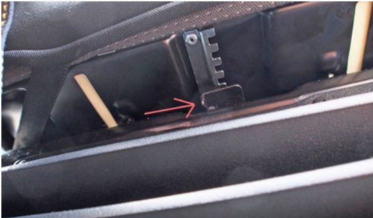
push lever in direction indicated by arrow,
