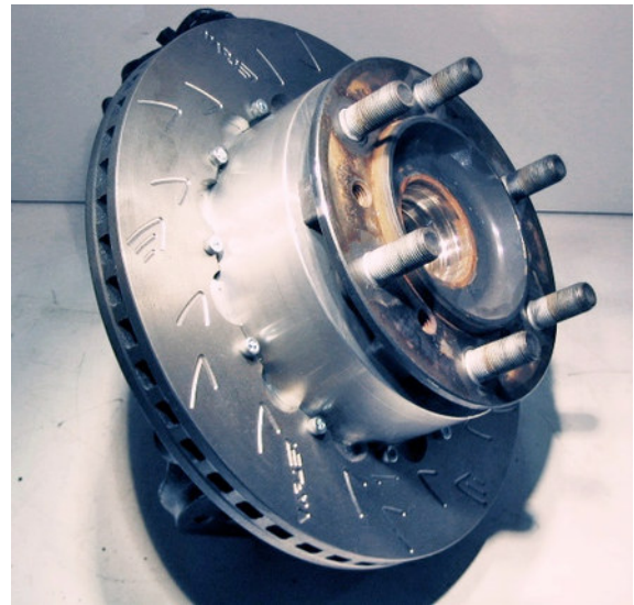
Bell (mounting hat) bolted to hub
