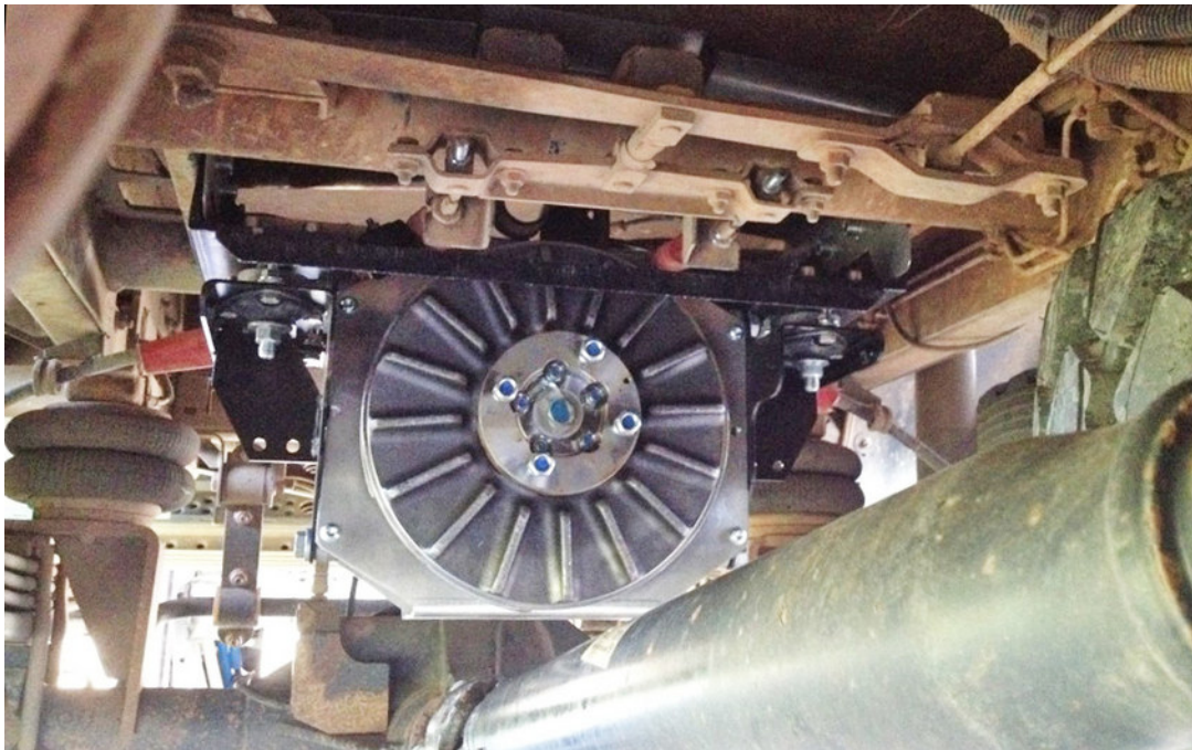
Retarder mounted in the chassis
