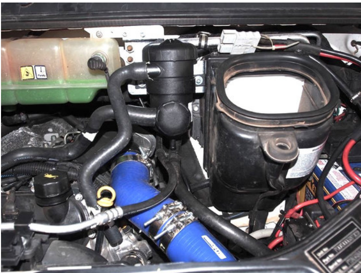
Provent 200 PCV unit installed on firewall
