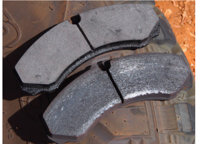
new softer LPR pad vs 15,000km IVECO "metallic pad"
