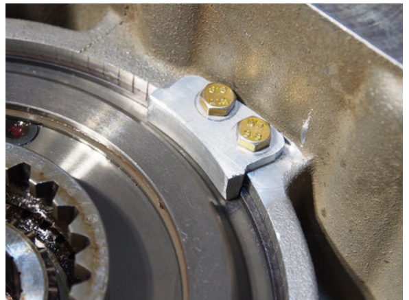
Circlip 'lock' makes sure it can never pop out
