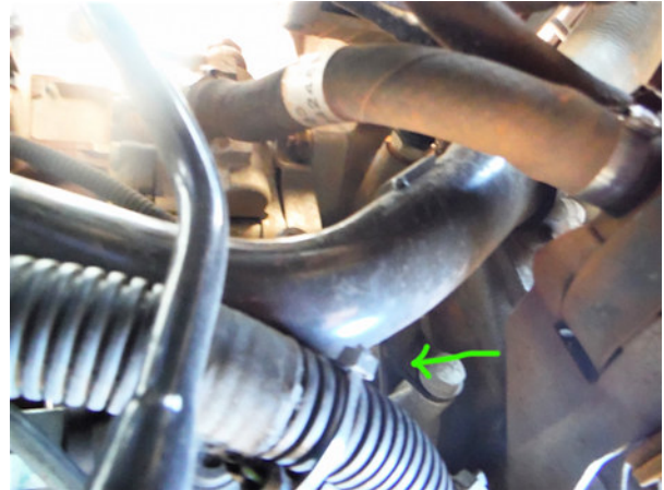
CableTie tang too close to coolant hose
