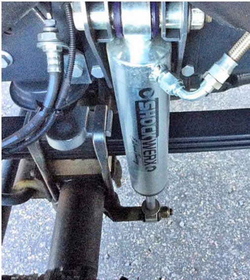
Shock Werx remote reservoir gas shocker
