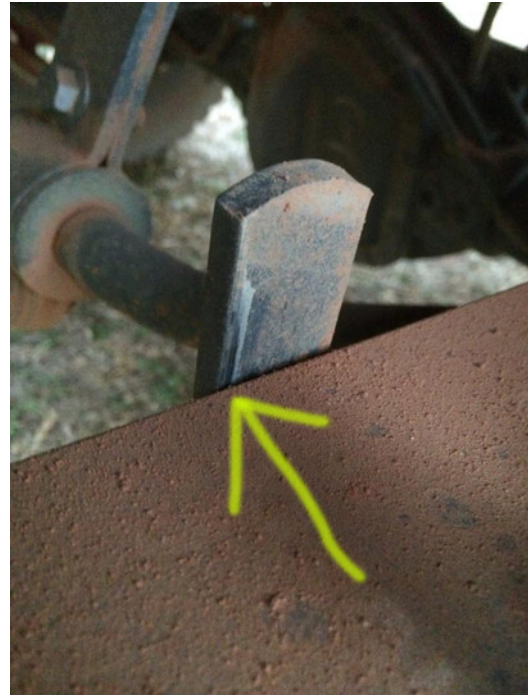
evidence of rubbing
