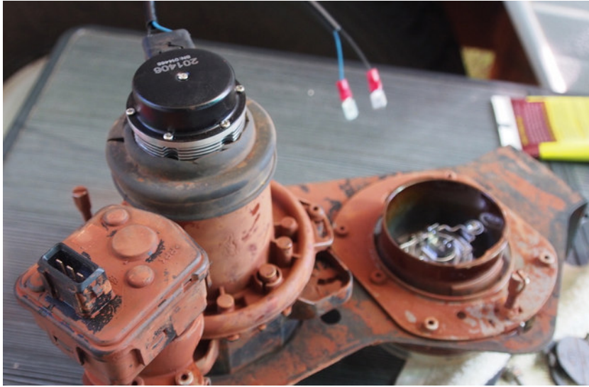
H7 LED mounted in Hella housing
