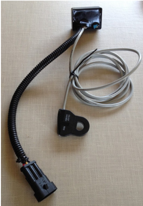
ABS power cable through current sensing module
