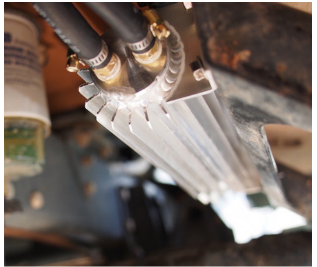
Dual Pass 12" finned alloy transmission cooler makes a great fuel cooler, fits under dual cab rear step
