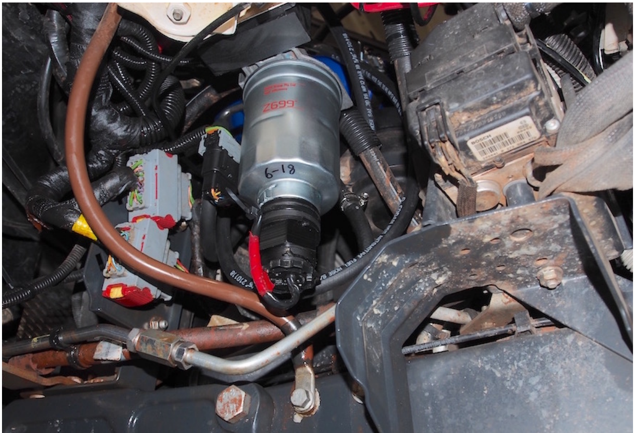
LandCruiser CRD Z699 spin on filter with Iveco sensor adapted.
