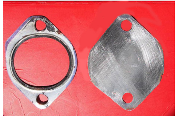
EGR gasket and "full" blanking plate
