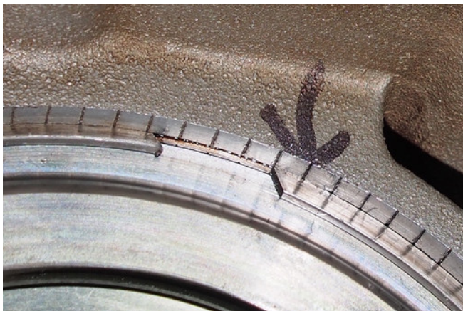
less than 0.9mm of circlip sits in the groove
