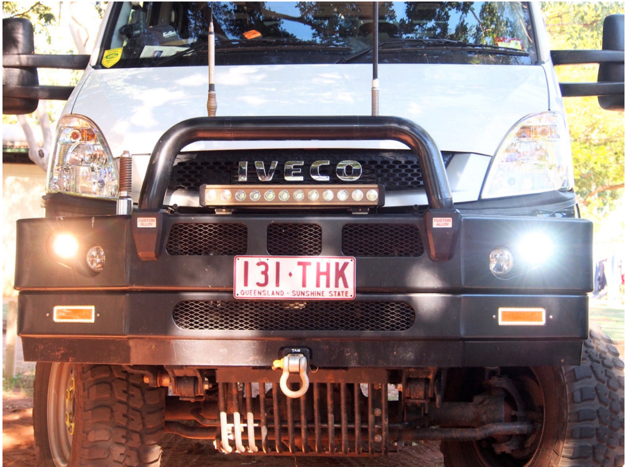
comparison showing original H7 Halogen bulb driver side versus H7 LED bulb .
