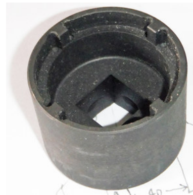
TC nut tool Iveco part no 99355047
