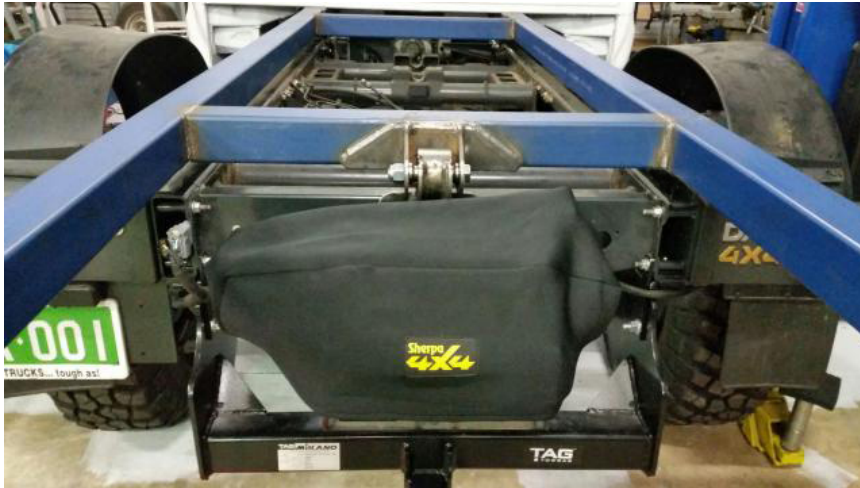
rear of EVA 3-point mounting system
