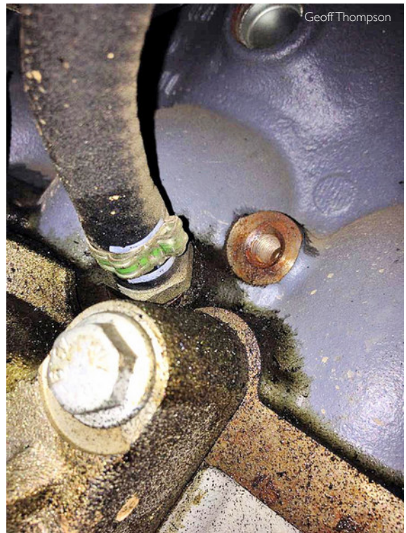
top (small) turbo drain hose
