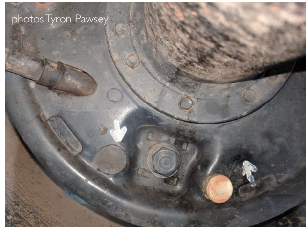
Left side , and right side rear backing plates, note new rear shoe adjuster holes with corks
