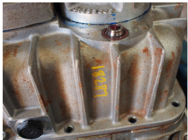
External oil seal in place of selector shaft o-ring
