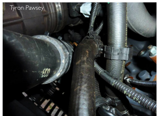
fixed using rubber shroud around hose
