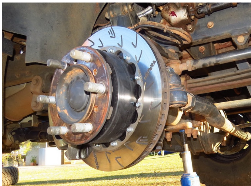
original ABS tone ring re-fitted
