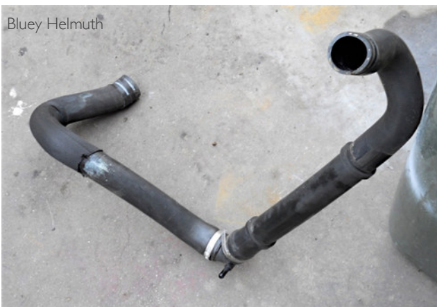
Radiator hose / Cable Tie rub through
