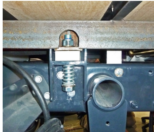
Traveltrucks kinetic mounting system uses multiple sprung mounts.
