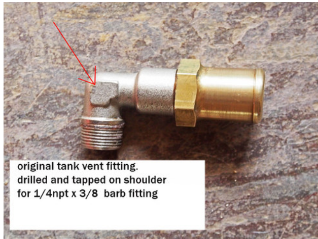
examples of hose adaptors used to plumb aux tank into original tank fittings
