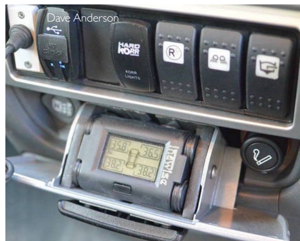
"Inawise" TPMS fits neatly into Ash Tray
