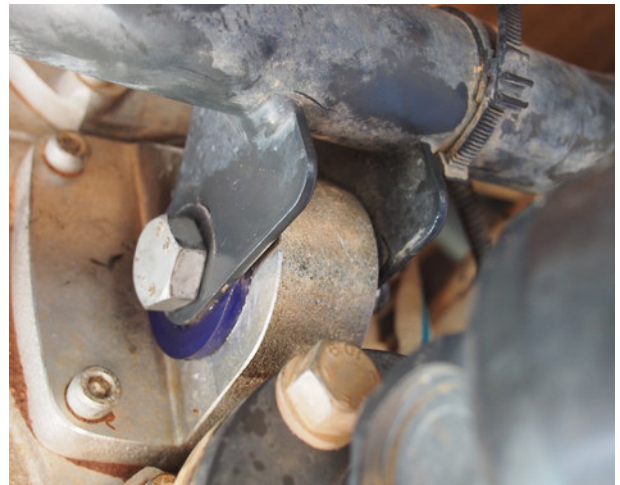
cut in half for insertion from each side
