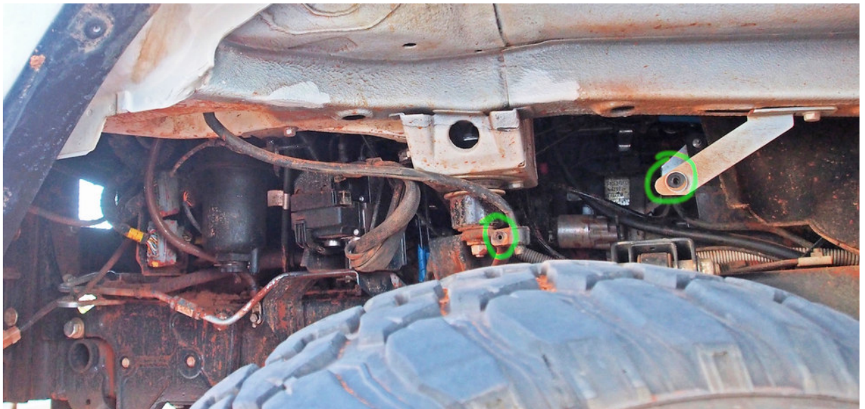
left inner guards removed, same fixing points highlighted
