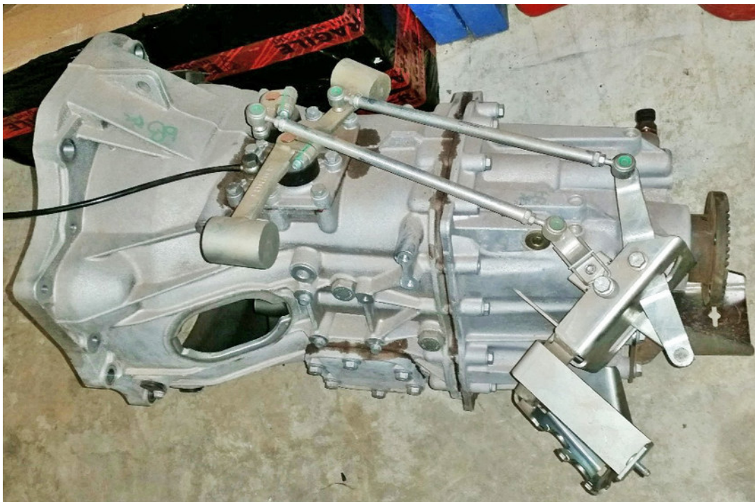
ZF 6S 400 OD as removed from 55S17W
