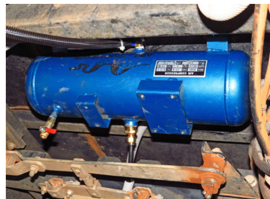
receiver mounted under tray
