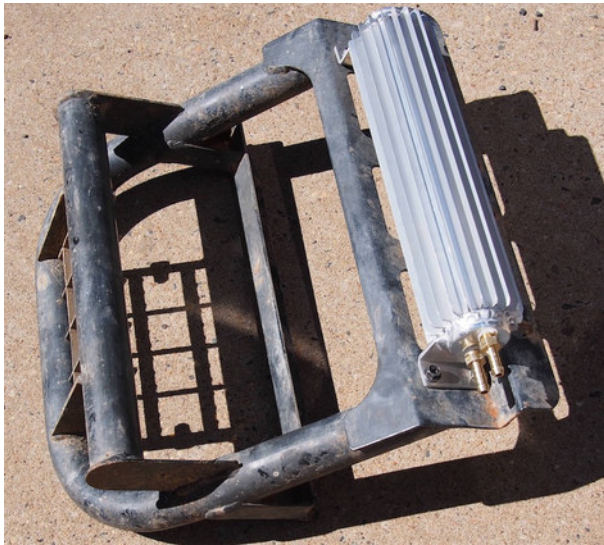
Dual Pass 12" finned alloy transmission cooler makes a great fuel cooler, fits under dual cab rear step
