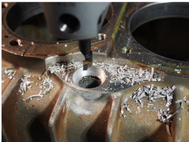
Boring out case to accept external seal
