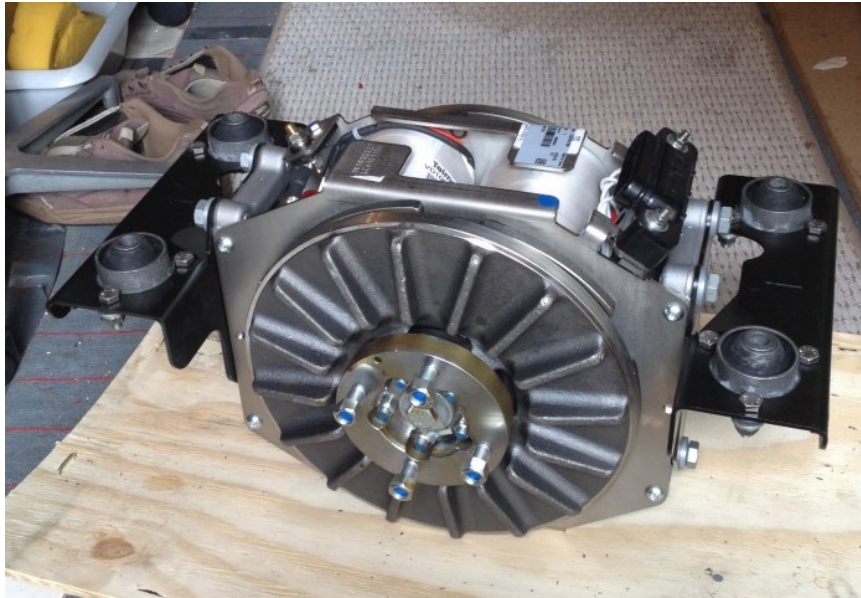
Retarder with Telma supplied brackets
