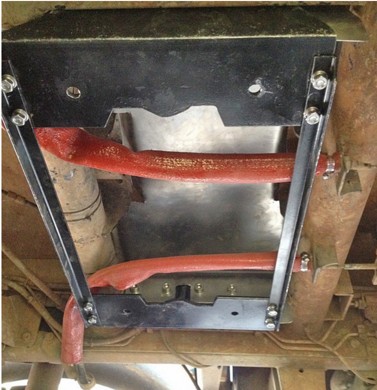
Bracket fitted with top heat shield and fire sleeve on handbrake cables
