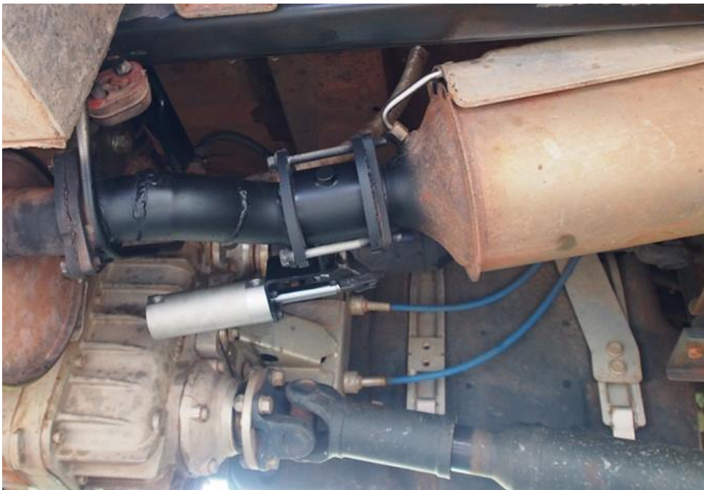
Gearing Dynamics 3" Exhaust Brake valve fitted to 55S17W
