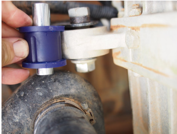
one full poly-bush with cut off flange
