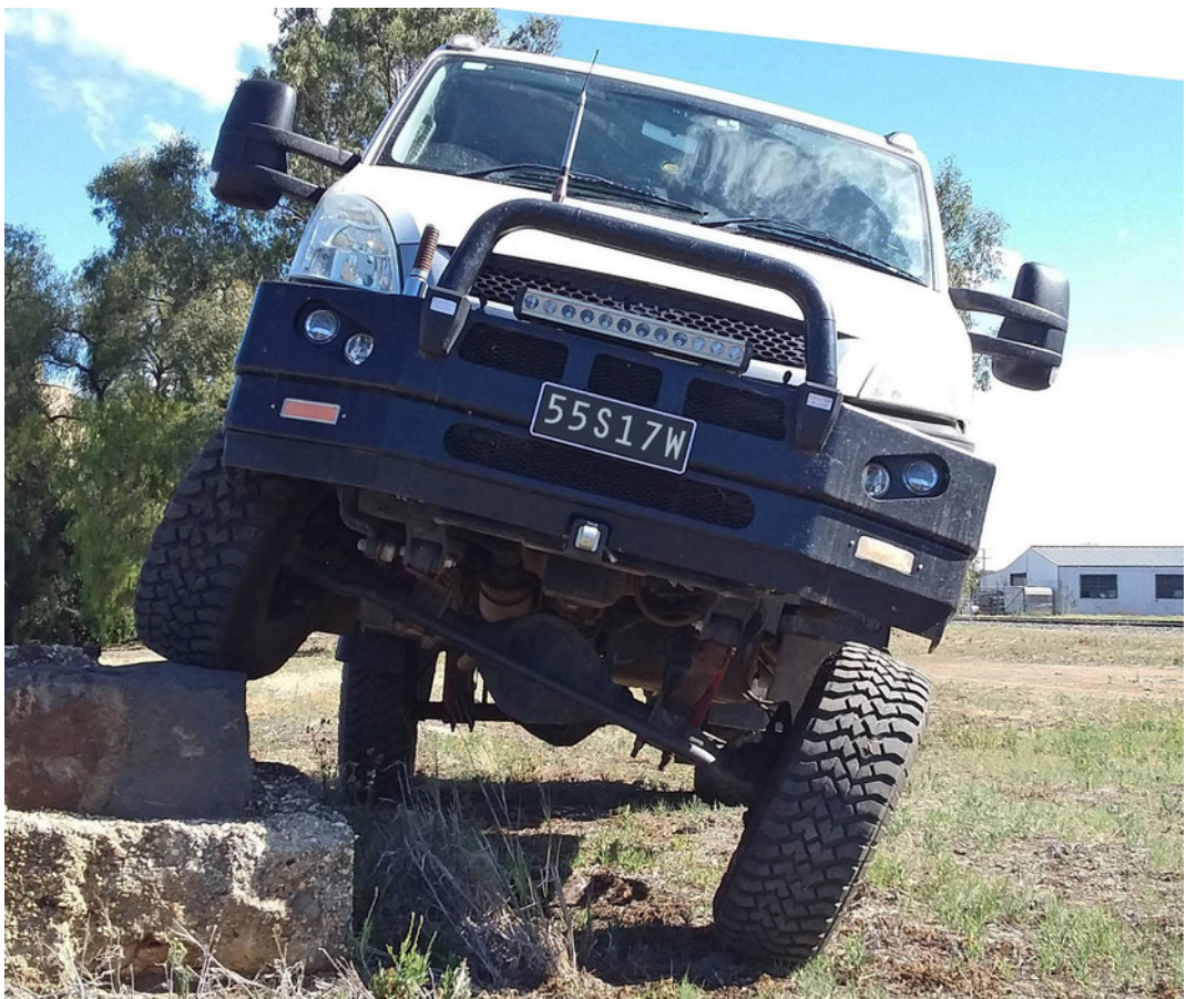
Standard suspension with front roll bar removed (for off road use only)_
