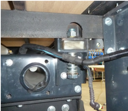
Traveltrucks kinetic mounting system uses multiple sprung mounts.
