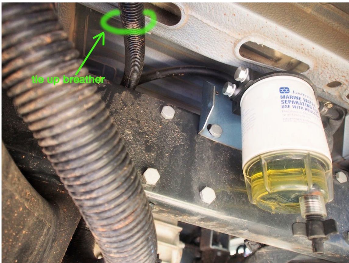
Aftermarket Racor style pre-filter - sedimenter
