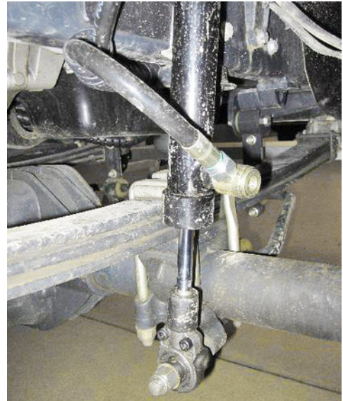
Citroen style hydraulic / accumulator
