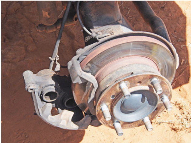
same truck, 60,000km , clearly needs a rotor grind
