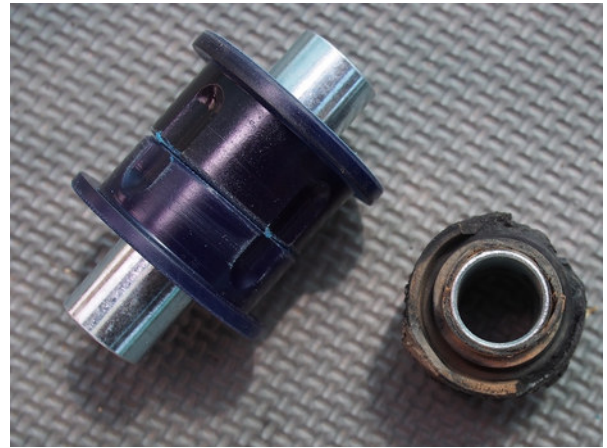
cut in half for insertion from each side
