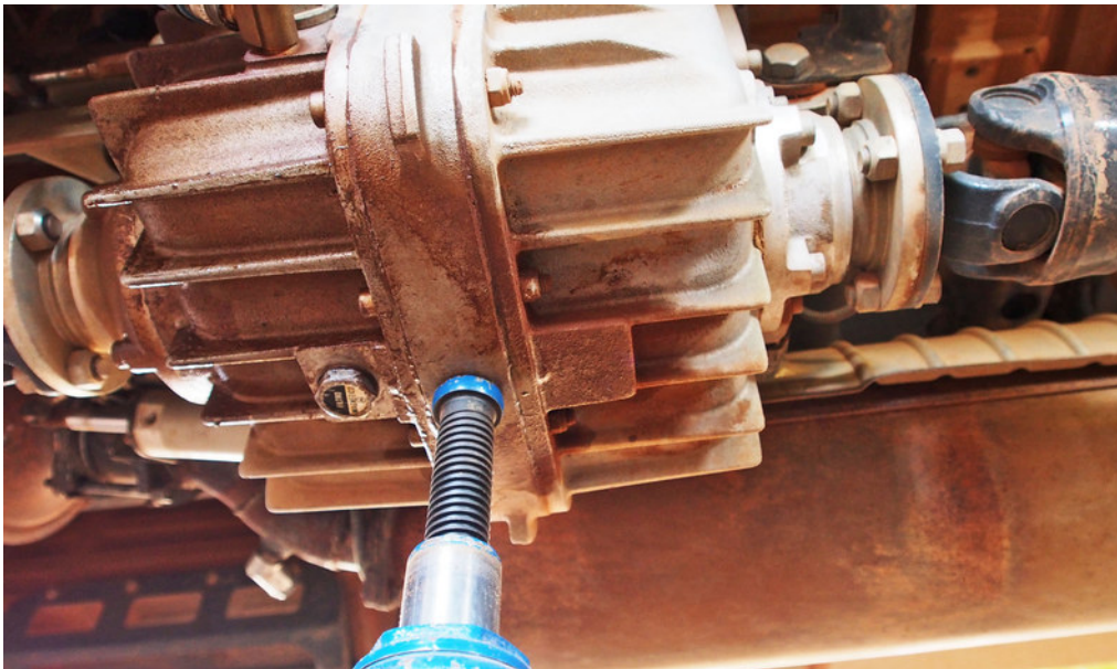
for examining TC bushes only, position jack in this location
