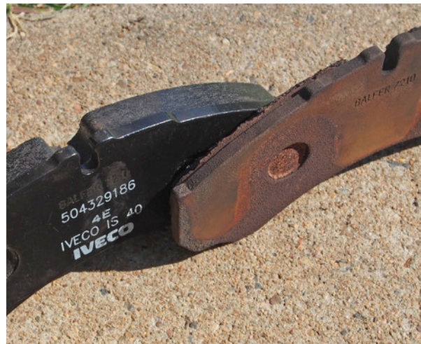
new vs pad passed as serviceable by dealer
