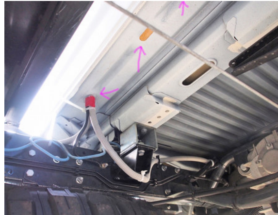
possible cable entry holes under rear floor
